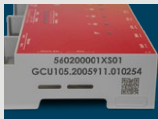
Laser printing of incremental QR codes/barcodes and serial numbers
